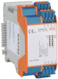
The Remote I/O Module ANTARES 4 Analog In/Out or 4 Analog In/Out HART is suitable for the direct connection of four intrinsically safe 2-, 3-, 4-conductor transmitters (4 to 20 mA) or for outputting 0 to 20 mA signals for analog actuators.
